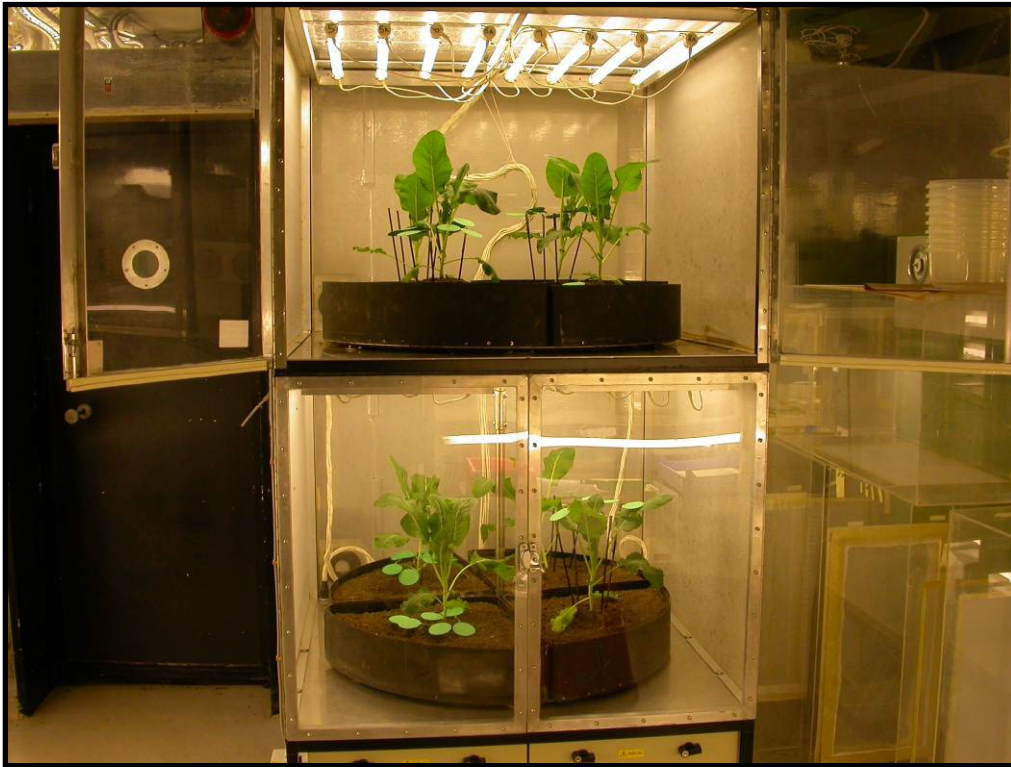
Figure 24. Rotating cage showing the two compartments into which test insects are released.
